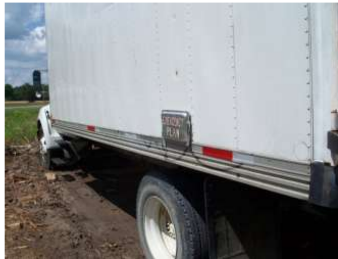
Fig. 1: Waterproof "manifest box" is attached to the body of the crew's service truck.
