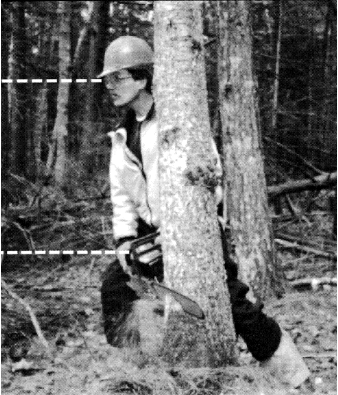
The site line on the saw can be used like a gun sight to determine an exact falling direction for the tree.
