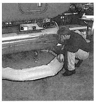
This inflatable spill protection pool from Ultra Tech, Inc. is an example of one of the many tools that can be used to prevent and/or minimize spills.
