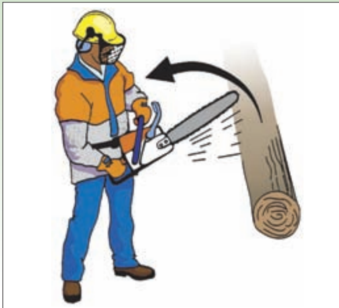
Dangerous kickback occurs when the front, upper corner of the tip of the bar on the chain saw comes in contact with an object.
